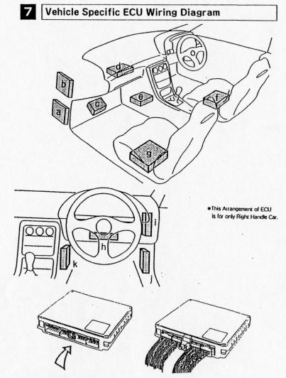
\*The Following Diagrams View the Coupler form the Same Angle as the Diagram Please be Careful Not to make Improper Connections or Short Out the Unit.
